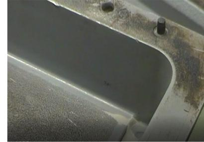
Fig 1. Dirty mould inlaid with material from the production process.
